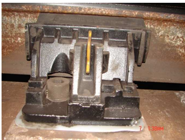
Figure 2 Pandrol VANGUARD low stiffness fastener
